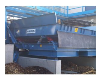
Spillage bark and wood waste are loaded by a front loader on a Vibrating Feeder Deck, feeding the material into the vibrating conveyor. Further transport of the processed bark is done by two TUBULATORs type CT500, length 50 + 100m.
